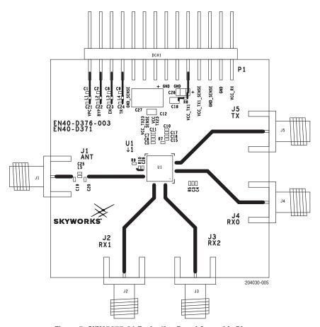
Figure 5. SKY65377-21 Evaluation Board Assembly Diagram
