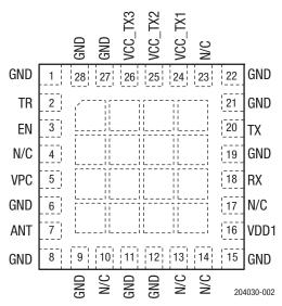
Figure 2. SKY65377-21 Pinout (Top View)
