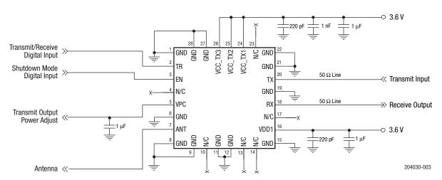
Figure 3. SKY65377-21 Typical Application Schematic
