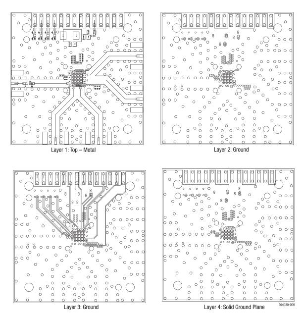
Figure 6. SKY65377-21 Evaluation Board Layer Detail
